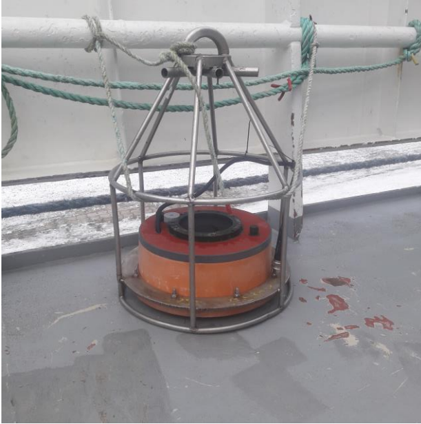
Fig. 8. Echo sounder mounted in a frame on board 'Vendla'.
