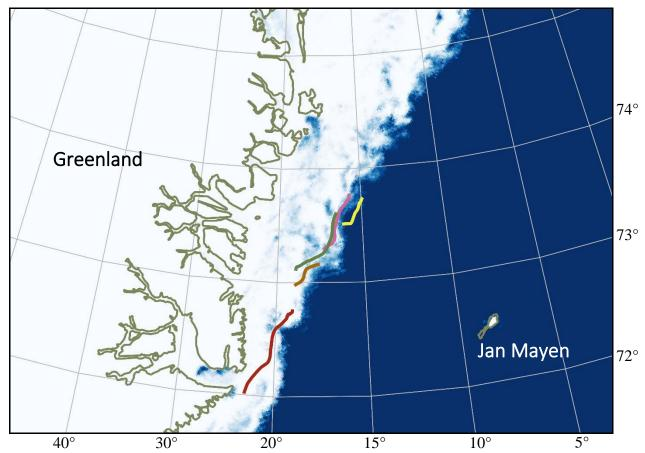
**Fig. 8**. Tracks of five GPS/Idirium tracking devices deployed by helicopter from KV Svalbard on ice floes around the main seal concentrations 18-24 March 2018. The tracks illustrated the ice drift up to and including March 24. The background image shows the sea ice concentration on 22 March (taken from the AMSR2 Sea Ice Concentration product, Spreen et al., 2008).
