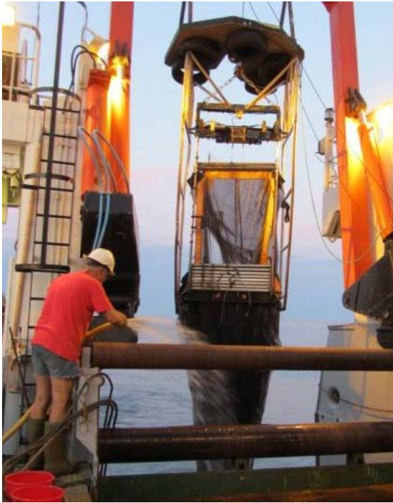
MOCNESS: Multiple Opening Closing Net with Environmental Sensors
