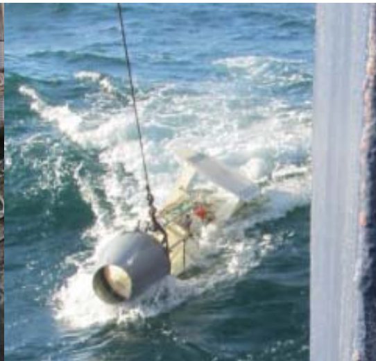
Gulf VII High-speed sampler with PUP net
