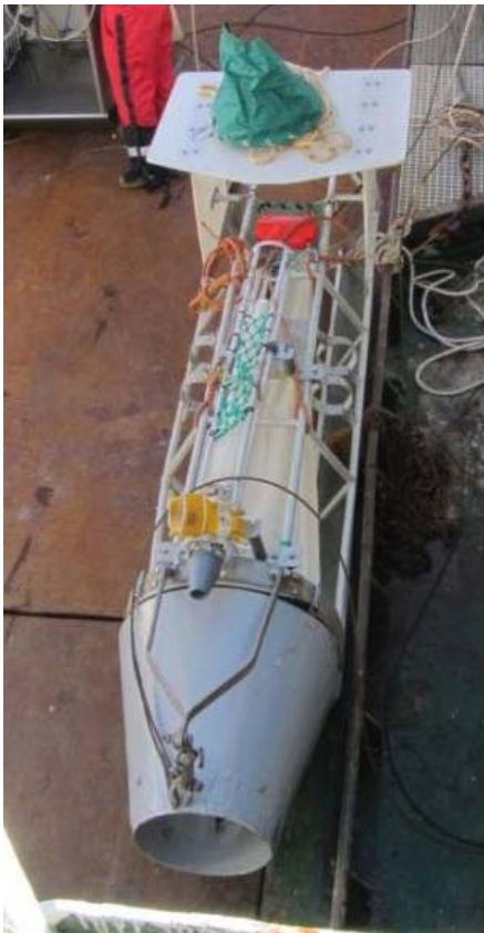
Gulf VII High-speed sampler with PUP net
