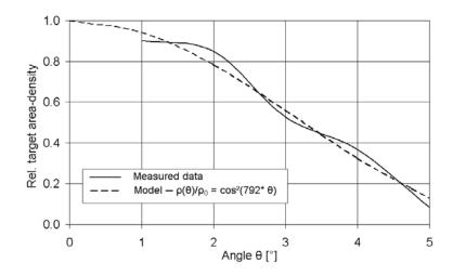
Figure 10. Relative area based target density within the beam of the transducer as a function of the angle  $\theta$ .
