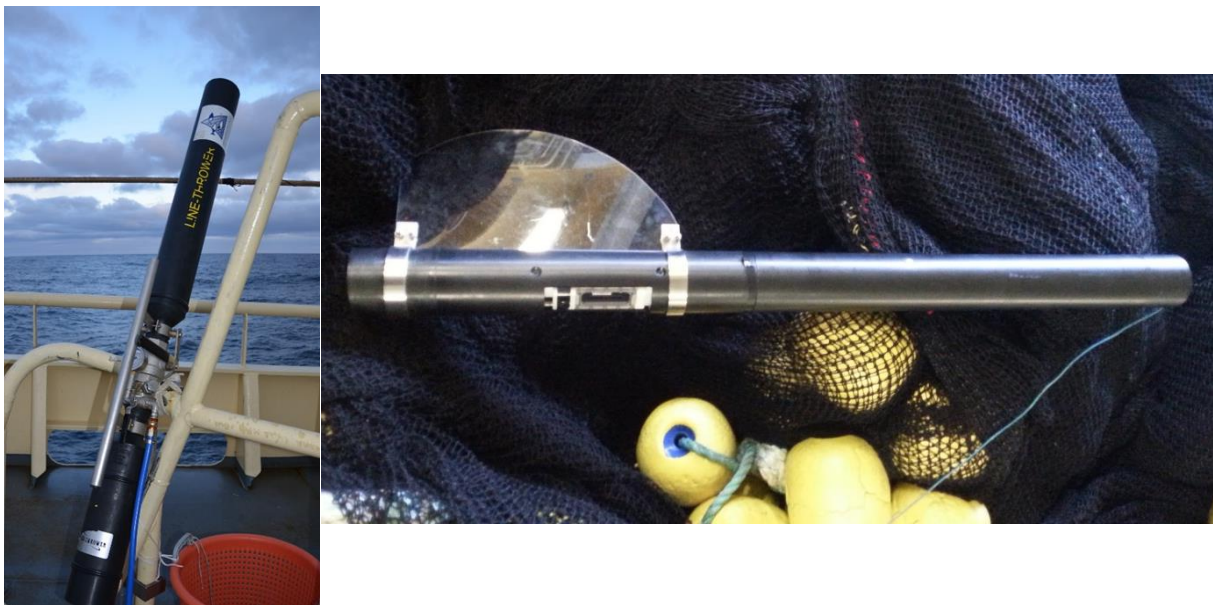
Figure 4.1: Catch monitoring probe (CMP) in protective housing (right) prepared for deployment from a compressed air canon (left).
