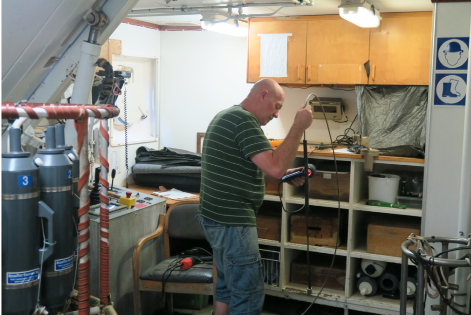
The Chief Instrument Engineer Tore Mørk is re-terminating the broken CTD cable.
