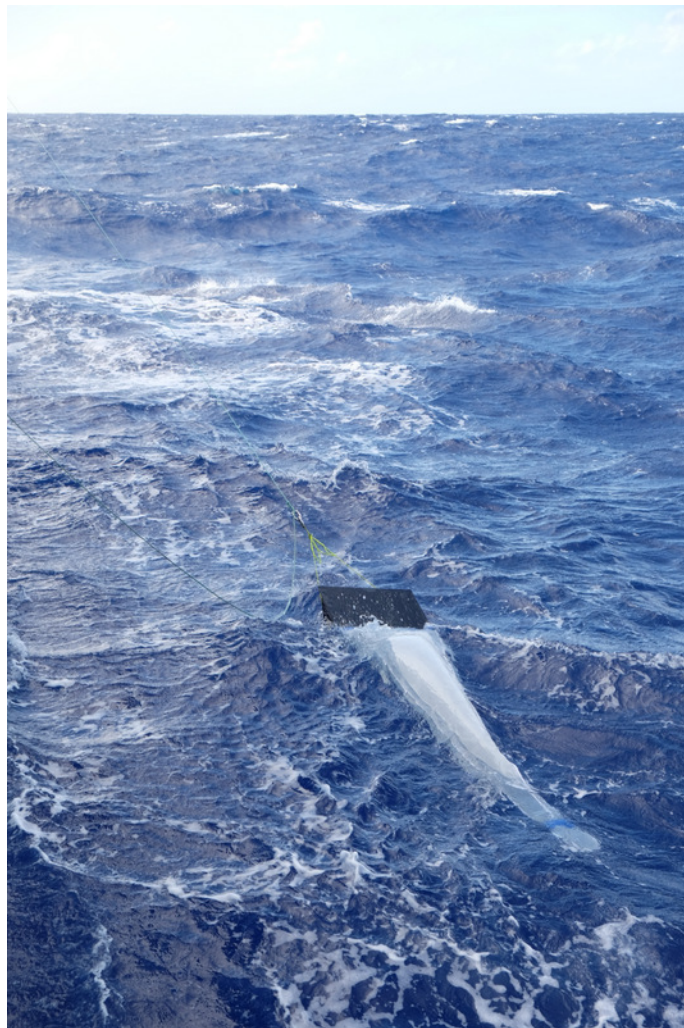
Manta-trawl for sampling of plastic particles in the surface.
