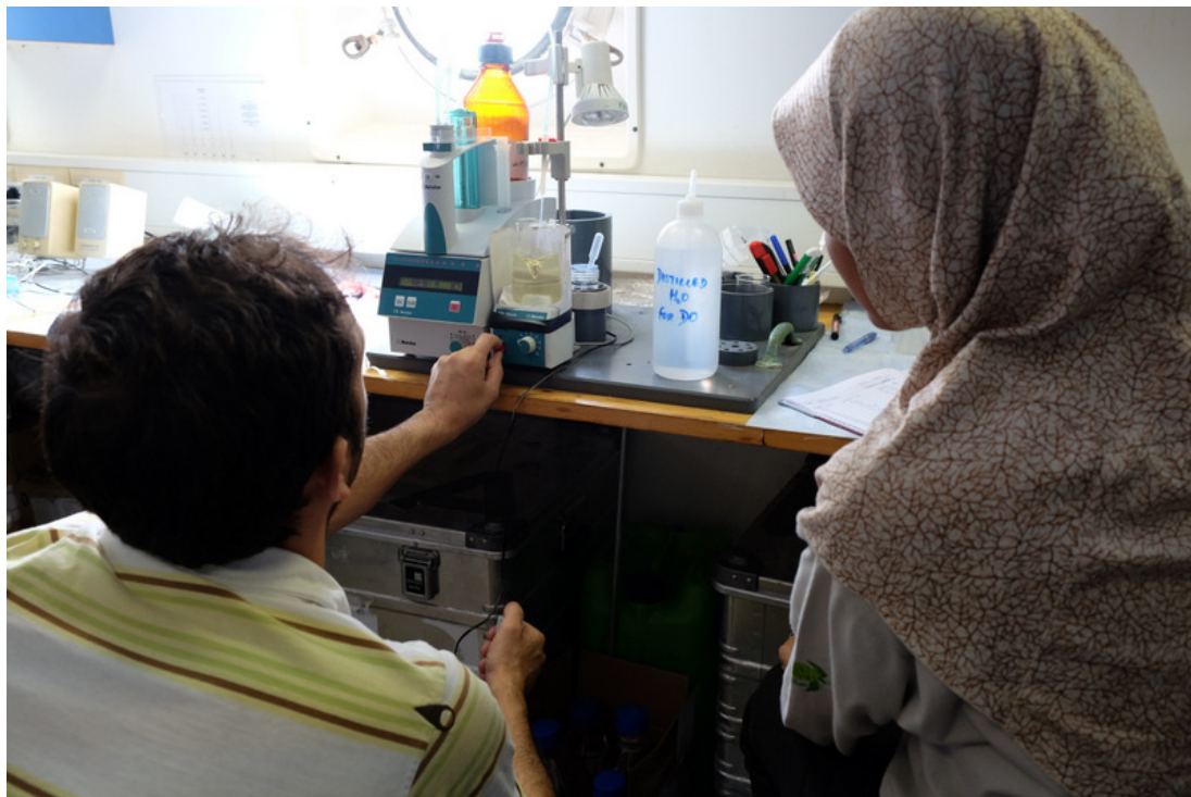
Doing analysis of the content of oxygen in sea water.
