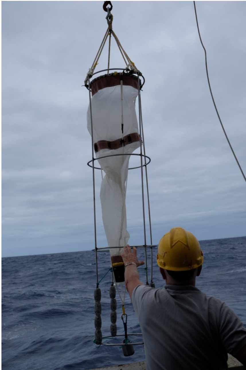
The net for sampling of phytoplankton. The net has a mesh size of 10 \mu\text{m} only.
