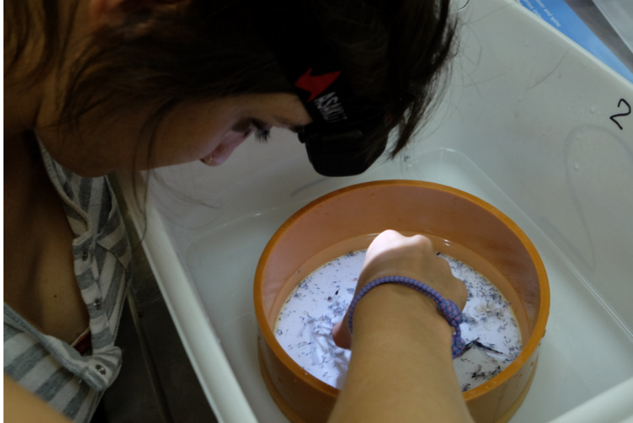
Sorting samples from the Manta trawl for plastic particles.
