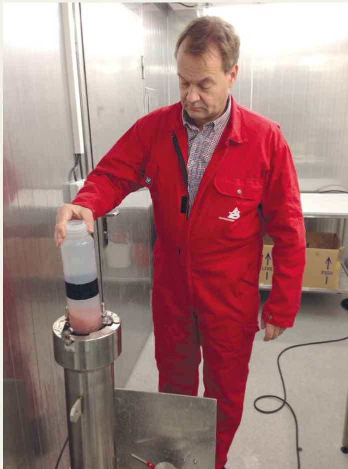
Figur 1. Eggene senkes i trykkcellen hvor de skal holdes på 655 bar i 5 minutter. The eggs are lowered into the pressure cell to be held at 655 bar for 5 minutes.
