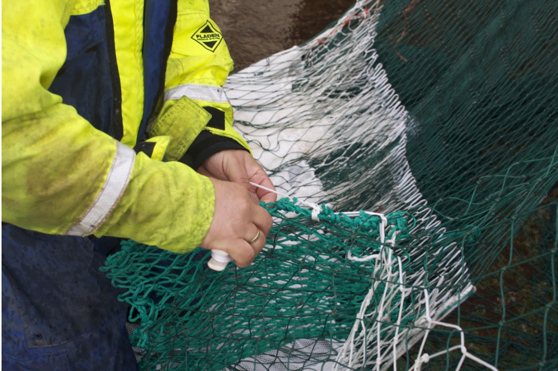
Figure 2. Front part of the inner net mounted to the 120 mm mesh of the trawl net itself.
