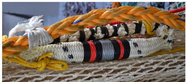
Figure 17 – a depth sensor (D-0130) in its protective housing and sheath fixed to the top of the CCR.
