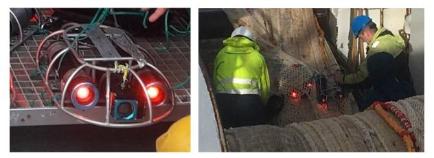
Figure A1 – "dome-frame" with camera (in a B-group housing), and with two red lights (left), and being fitted/removed from the trawl (right).
