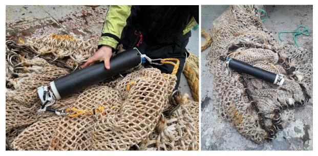
Figure 23 – Rinko oxygen logger, inside protective housing, being fitted inside the codend skirt before was coupled with the fish pump during Haul 03.
