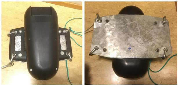
Figure A2 – the JT Electric Trawl Camera (Left), with a reinforcing base-plated fitted by the Vikingbank's engineers during the cruise (right).
