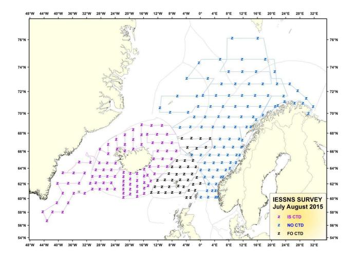
**Figure 2.** CTD stations (0-500 m) using SEABIRD SBE 37 (Arni Fridriksson, purple) SEABIRD SB 25+ (Christian í Grótinum, black) and SAIV SD200 (Brennholm and Eros, blue) CTD sensors and WP2 plankton net samples (0-200 m depth). These were taken systematically on every pelagic trawl station on all four vessels.
