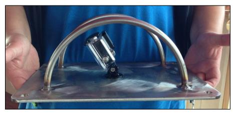
Photo 1. GoPro camera inside a waterproof box, mounted on steel frame and ready for employment in trawl on Finnur Fríði.
