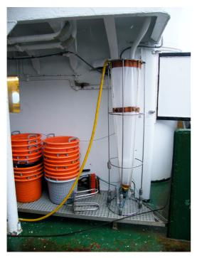
Experimental net haul: running sea-water through the algae-net upright on the rear deck.
