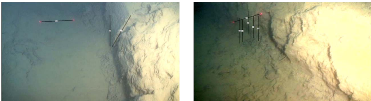
Figure 24. Tracks of door from the rockhopper trawl. The black bars shows measurements done to size the track. The distance between the red laser lights was 10 cm.
