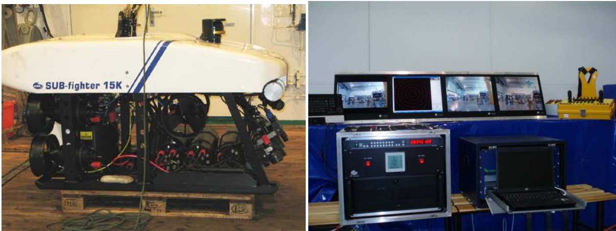
Figure 13. The ROV Subfighter 15K (left) used for bottom habitat mapping. The right picture shows the surface control equipment and observation screens.
