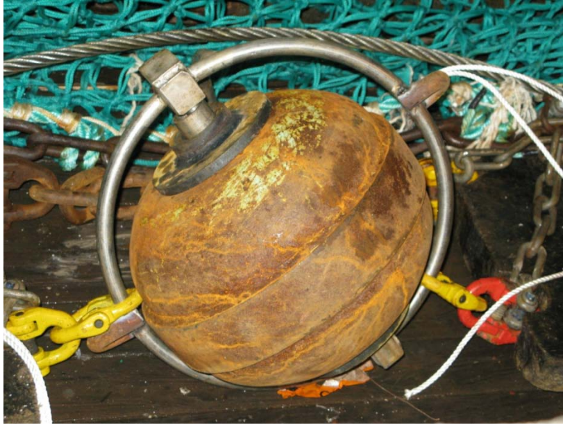
Figure 12. One of the bobbins specially designed to always roll in the towing direction of the trawl.
