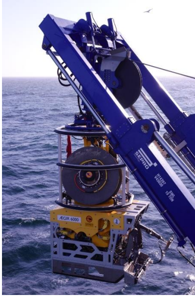
Figure 3.5. Launching of ROV Ægir 6000 at the 7 th of July, equipped with three 1 l biosyringes and two 2 l Niskin bottles. Dive 1.
