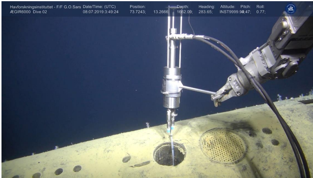
Figure 3.10. Collection of 1 l seawater inside the ventilation pipe with a biosyringe.
