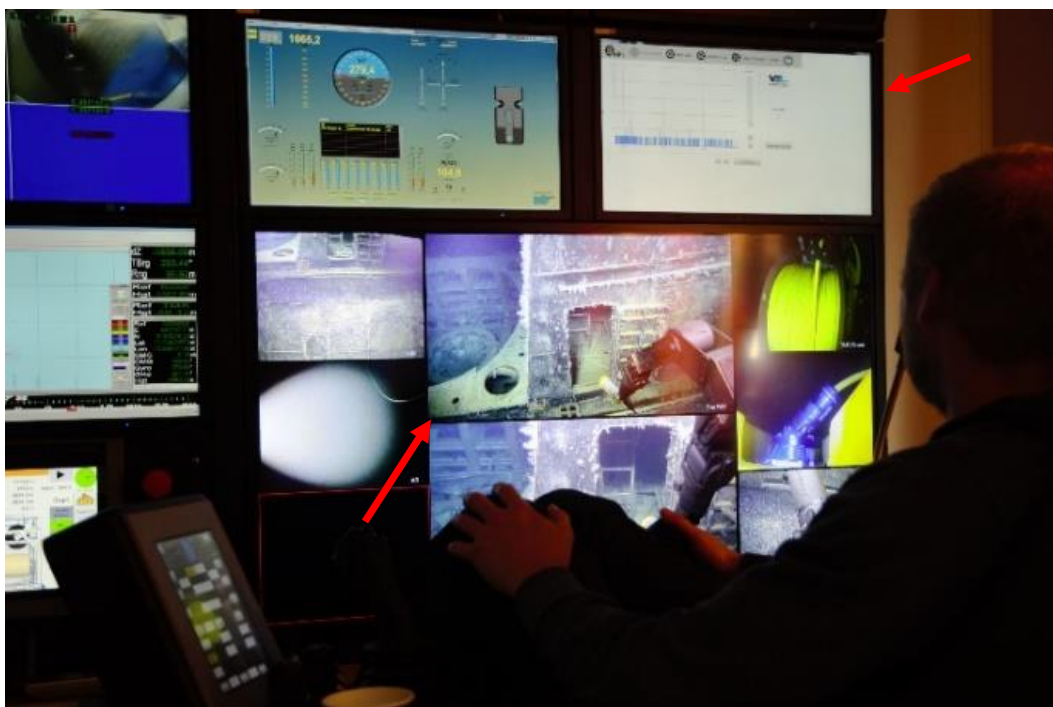
Figure 3.17. From the ROV control room onboard RV “G. O. Sars”. The left red arrow point at two screens showing the work of the ROV. When this picture was taken, the ROV was screening the hull of “Komsomolets” with the VEL Subsea Geiger counter (see Figure 3.16). The upper right arrow points at the specter of the VEL Geiger counter. The VEL Geiger counter did not detect any radioactive contamination around the wreck of “Komsomolets”.
