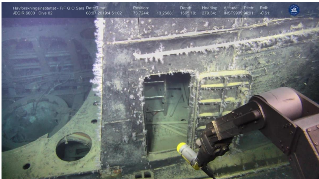
Figure 3.16. Screening of the tower of “Komsomolets” with the VEL Subsea Geiger counter (yellow instrument). The left part of the picture shows the area where the escape capsule originally was mounted.
