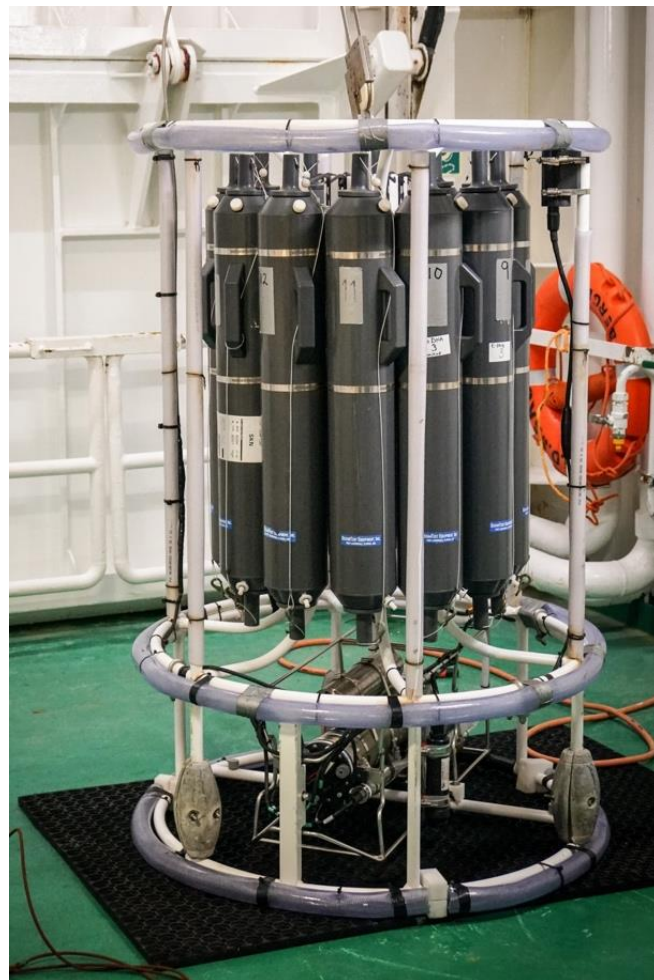
Figure 3.2. The CTD system onboard RV “G. O. Sars”. Photo: Stine Hommedal/IMR.
