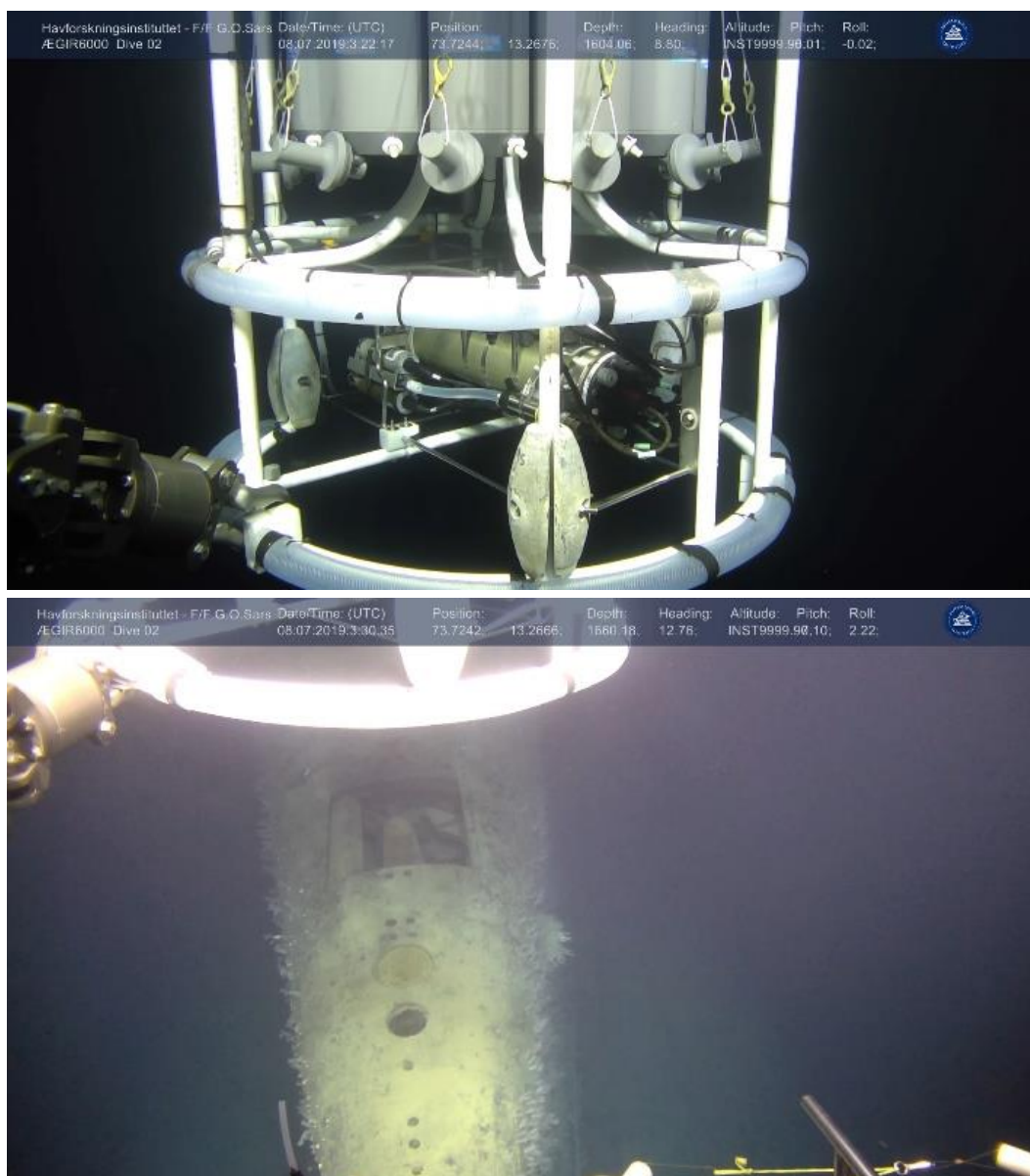
Figure 3.8. Sampling of seawater 3 m above the ventilation pipe. The ROV Ægir 6000 brought the CTD system/Rosette Sampler to the desired position for sample collection (the ROV arm is visible in the left part of the picture).
