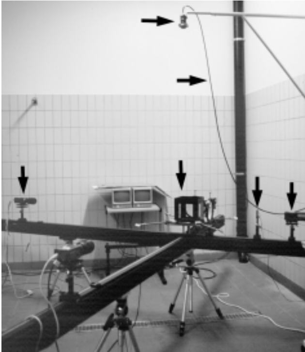
Figur 1 Silhouette video photography system (SVP) used to make behavioural observation of fish larvae. Light from a 1-kW Xenon arc lamp (not shown) is focussed onto the aperture of a UV-visible liquid light guide (O) and passes through various optical components in a filter holder (F) before reaching the test aquarium (A) in which the animals are freely swimming in 12 l of sea water. The aquarium (30 cm square) is located at the intersection of two 3 m long optical rails. Each rail supports a far-red light emitting diode (D) placed at the focal point of a 14.5 cm diameter biconvex collimating lens (L), and a video camera (C) to image the shadows projected by the collimated beam that passes through the aquarium. Also shown are the lasers (Ar) that are used to align all of the optical components on the rails prior to a given set of experiments. The red spot at the far end of one of the rails is the light emitted by the diode.
