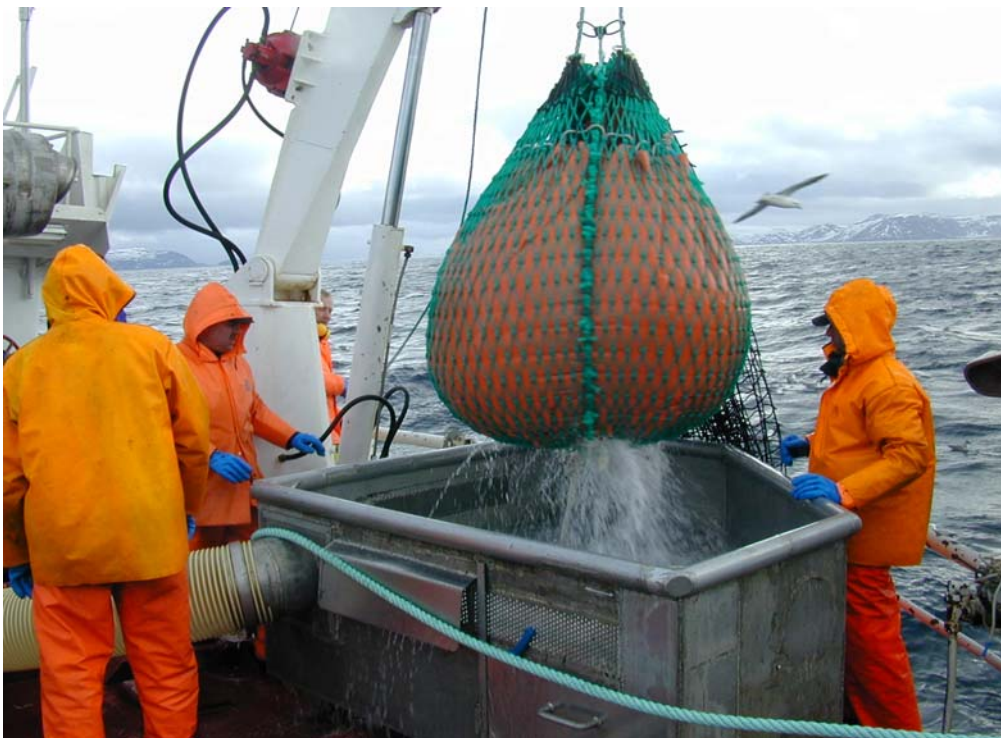
Bilde 3. Lerretsløft med fisk og vann heises om bord for tømning i sorteringskar. Picture 3. Lifting bag with canvas filled with water and fish ready for emptying on the sorting tray.
