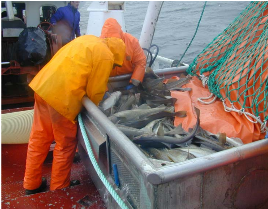
Bilde 4. Fisk sorteres, telles og slippes ned i føringsrom via en 14'' fleksibel slange. Picture 4. Live cod is sorted out, counted and transferred to the waterfilled hull through a 14-inch flexible tube.
